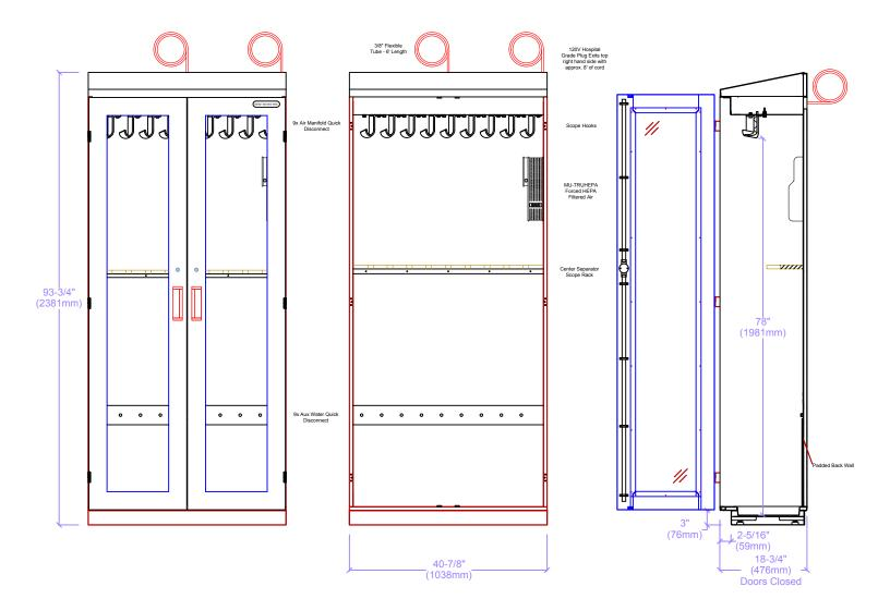
Item STAINLESS STEEL METAL CABINET SAS-9S-HA Capsa METAL SCOPE CABINET Locking Overlay Hinged Doors with Glass Inserts & Sloped Top, Holds 9 Flexible Endoscopes
