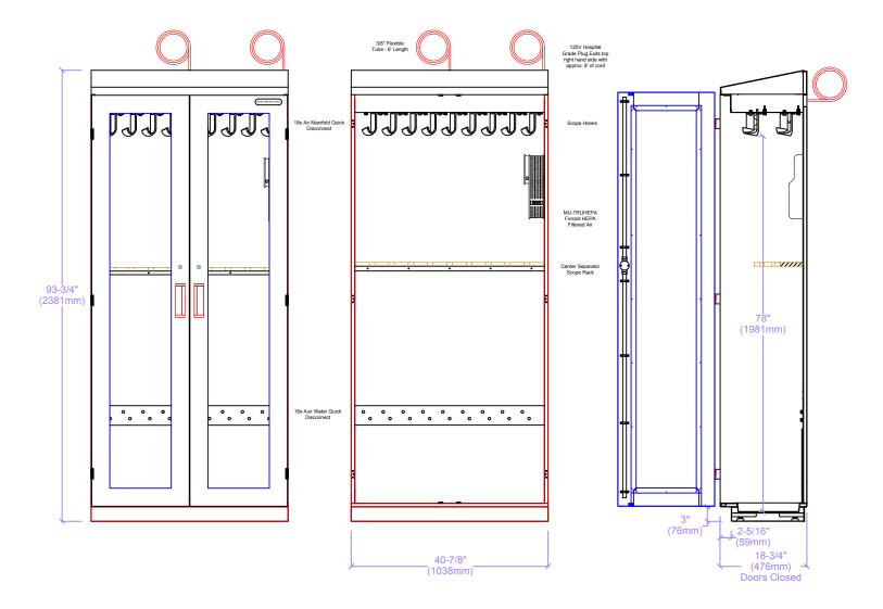
Item STAINLESS STEEL METAL CABINET SAS-18S-HA Capsa METAL SCOPE CABINET Locking Overlay Hinged Doors with Glass Inserts & Sloped Top, Holds 18 Flexible Endoscopes
