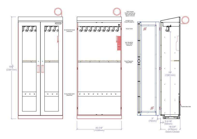
POWDER-COATED METAL CABINET SAS-9P-DRY Capsa METAL SCOPE CABINET Locking Overlay Hinged Doors with Glass Inserts & Sloped Top, Holds 9 Flexible Endoscopes
