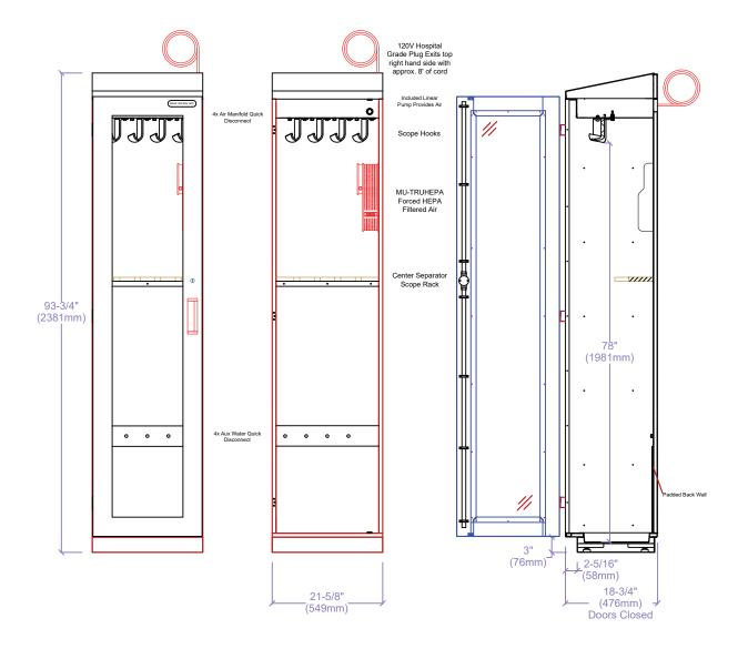
POWDER-COATED METAL CABINET SAS-4P-DRY Capsa METAL SCOPE CABINET Locking Overlay Hinged Doors with Glass Inserts & Sloped Top, Holds 4 Flexible Endoscopes
