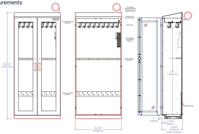
POWDER-COATED METAL CABINET SAS-18P-DRY Capsa METAL SCOPE CABINET Locking Overlay Hinged Doors with Glass Inserts & Sloped Top, Holds 18 Flexible Endoscopes
