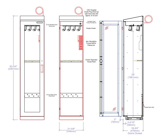
POWDER-COATED METAL CABINET SAS-8P-DRY Capsa METAL SCOPE CABINET Locking Overlay Hinged Doors with Glass Inserts & Sloped Top, Holds 8 Flexible Endoscopes
