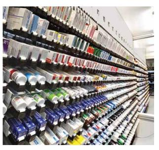
Replenishment is logical, fast, and uncomplicated. Technicians scan the medication's bar code, enter the quantity to load, and insert medication packets. RoboPharma software guides the replenishment and tracks inventory levels.
