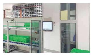
RoboPharma's operating system steers the network of high-speed dispensing robots and integrated tote conveyors so there is no holdup or backup to each hospital ward's mini-pharmacy.
