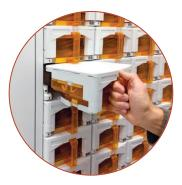
Cassettes can only be removed by an authorized user. Ideal for scheduled and high-value medications, and inventory control. Cassettes can only be opened while docked at the Cassette Station, and by an authorized user. FillSafe system prevents accidental mis-fills and unauthorized access.
