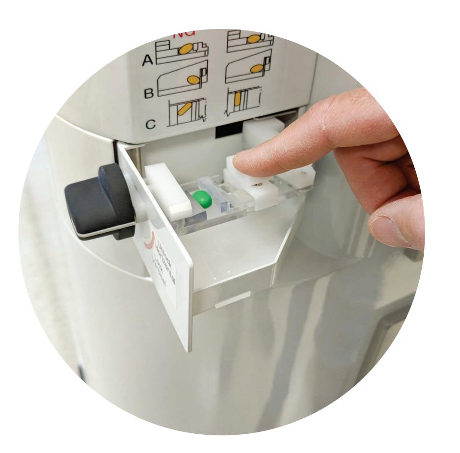
The KL108 camera chamber takes precise measurements of each new NDC/DIN to auto-calibrate the cassette.
