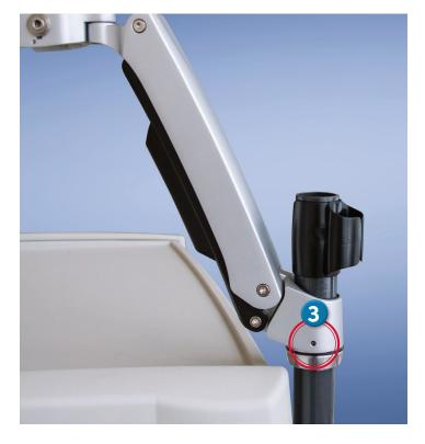
The rotational shaft pole screw adjusts the tension rotation of the articulating arm using the smaller Allen wrench provided. Turn counterclockwise for lighter tension (greater freedom of movement). Turn clockwise for tighter tension (less freedom or no freedom of movement).
